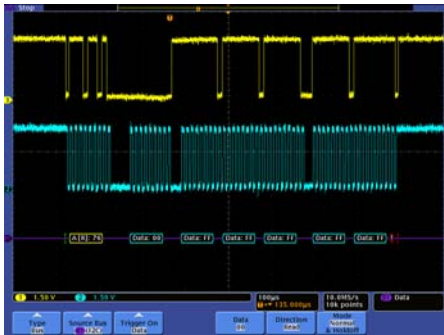
Triggering on specific data packet going across an I 2 C bus.
