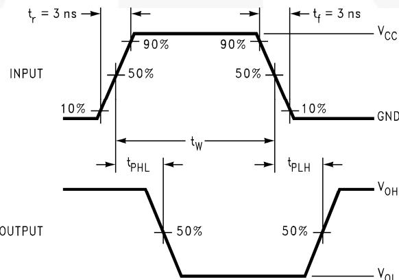
Figure 6. AC Waveforms
