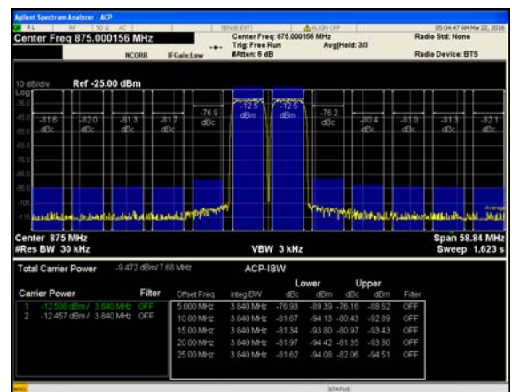
Figure 34. Two-Carrier W-CDMA at 875 MHz
