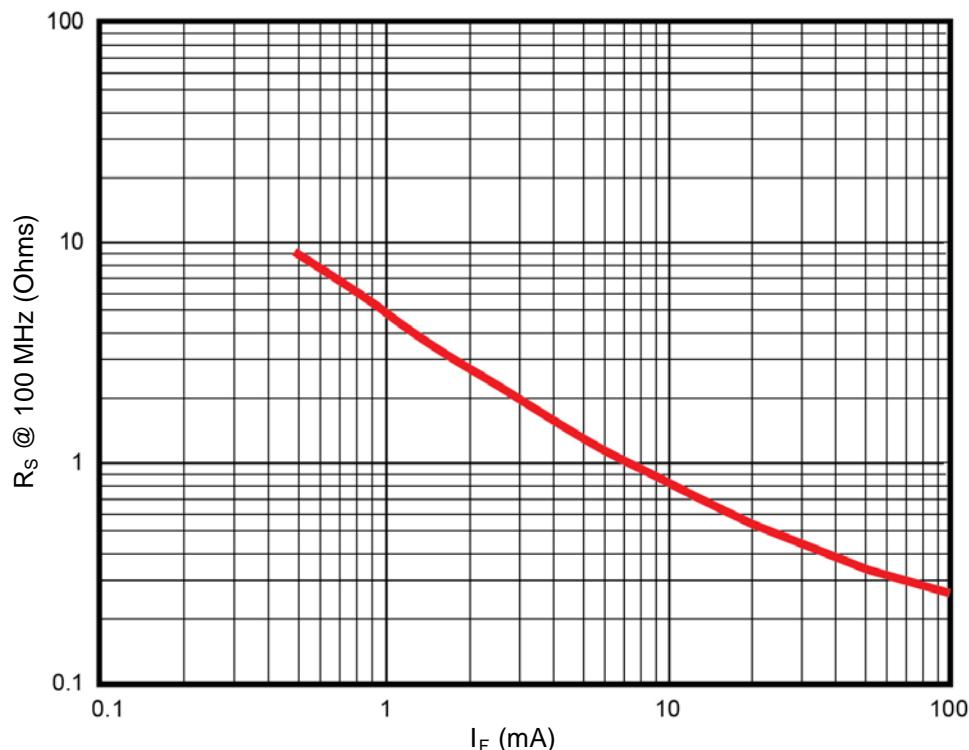
**FIGURE 1 - SERIES RESISTANCE (TYPICAL)**
