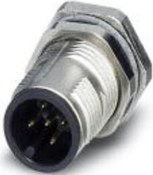
Sensor/actuator flush-type connector, 5-pos., M12-SPEEDCON, shielded, A-coded, rear/screw mounting with M12 thread, with straight solder connection
