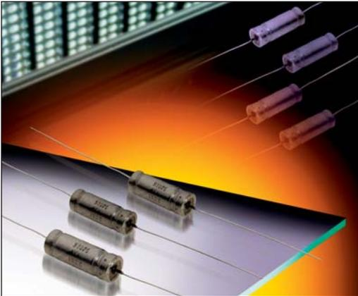
The TWA series is an axial leaded wet electrolytic tantalum capacitor and represents a new level of high CV (capacitance/voltage) previously unavailable in this technology. TWA incorporates a novel, very high capacitance cathode system that allows for higher CV designs, well beyond values specified in the Mil-PRF-39006 drawing.
