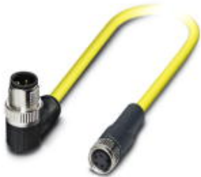
Sensor/Actuator cable, 4-position, PVC, Yellow RAL 1021, Plug angled M12-SPEEDCON, A-coded, on Socket straight M8, Cable length: 0.5 m
