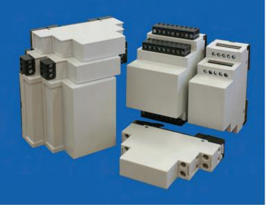
The versatile **KU4100 series** features a compact design with different terminal configuration options. They are available in six widths with double level terminal locations. Terminal configuration options include blank enclosures with no terminal openings, fixed PCB terminals and pluggable PCB terminals.
