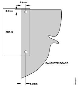
Figure 5. Maximum Board Dimensions for Connector Placement
