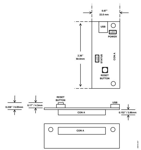
Figure 7. SDP-S Board Mechanical Specifications
