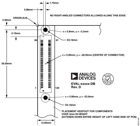
Figure 6. Connector Placement on Compatible Daughter Boards
