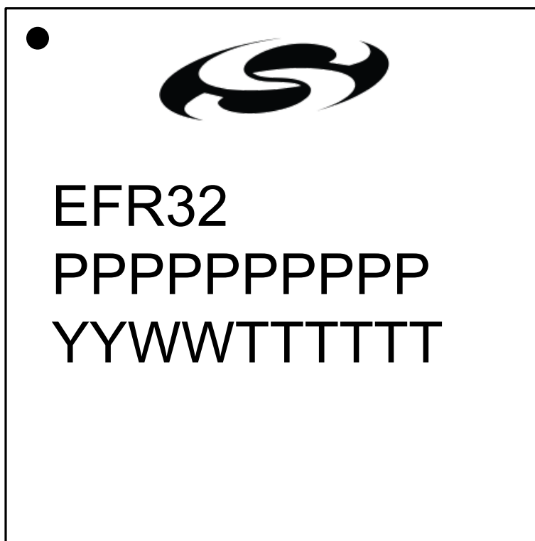
Figure 8.3. QFN48 Package Marking
