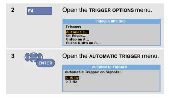
If the frequency range of the automatic triggering is set to > 15 Hz, the Connect-and-View™ function responds more quickly. The response is quicker because the test tool is instructed not to analyze low frequency signal components. However, when you measure frequencies lower than 15 Hz, the test tool must be instructed to analyze low frequency components for automatic triggering:
