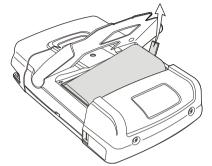
Figure 49. Removing the Battery
