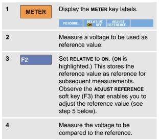
Now the large reading is the actual input value minus the stored reference value. The actual input value is displayed below the large reading (ACTUAL: xxxx), see Figure 13.
