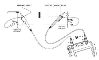
Figure 42. Correct connection of reference leads
