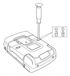
Figure 47. Unlocking the Battery Cover
