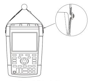
Figure 45. Fixing the Hangstrap
