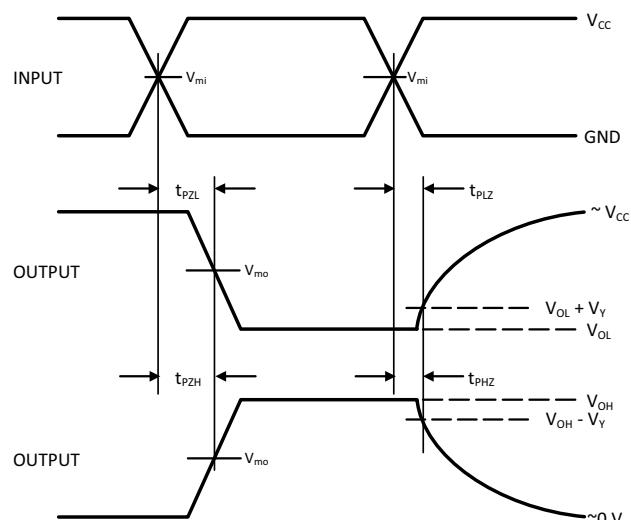
**Figure 4. Switching Waveforms**
