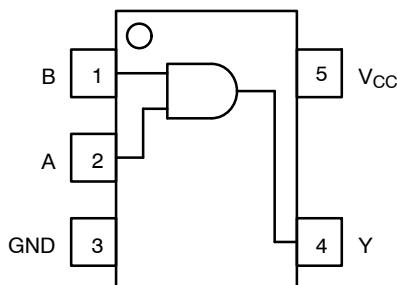
Figure 1. Pinout
