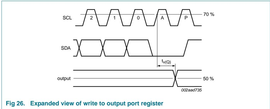
Fig 26. Expanded view of write to output port register
