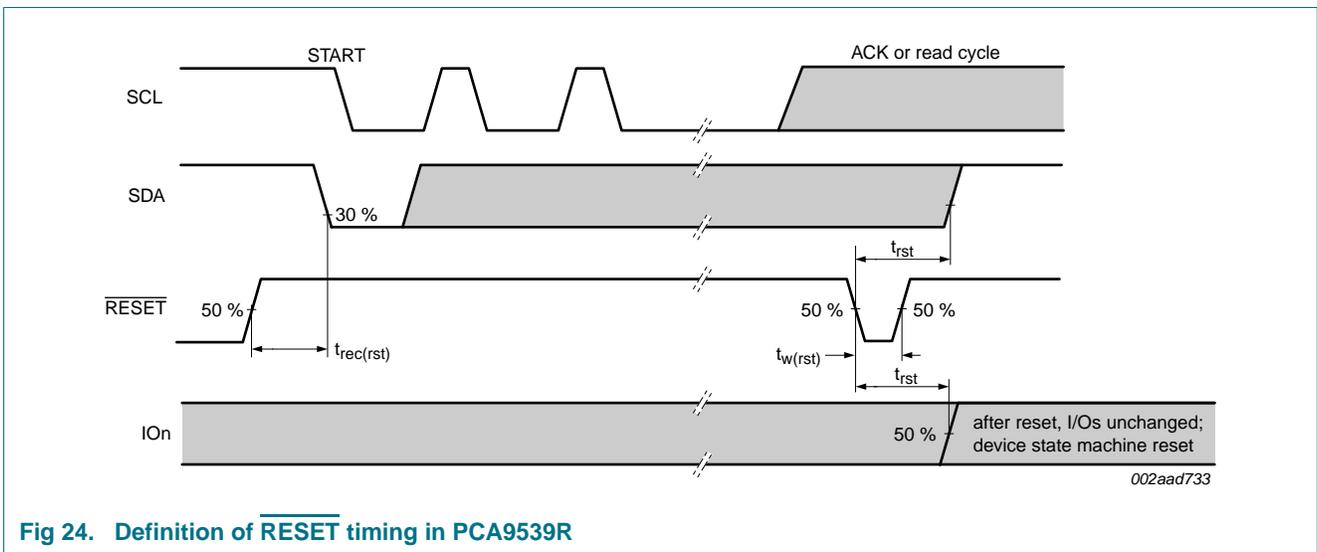
Fig 24. Definition of RESET timing in PCA9539R
