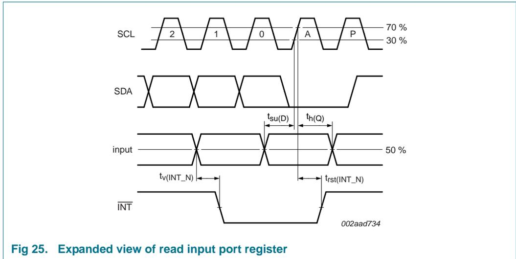
Fig 25. Expanded view of read input port register
