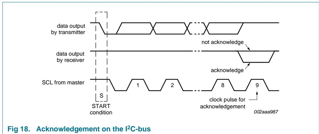
Fig 18. Acknowledgement on the I<sup>2</sup>C-bus
