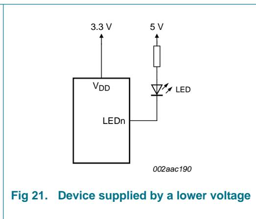
Fig 21. Device supplied by a lower voltage
