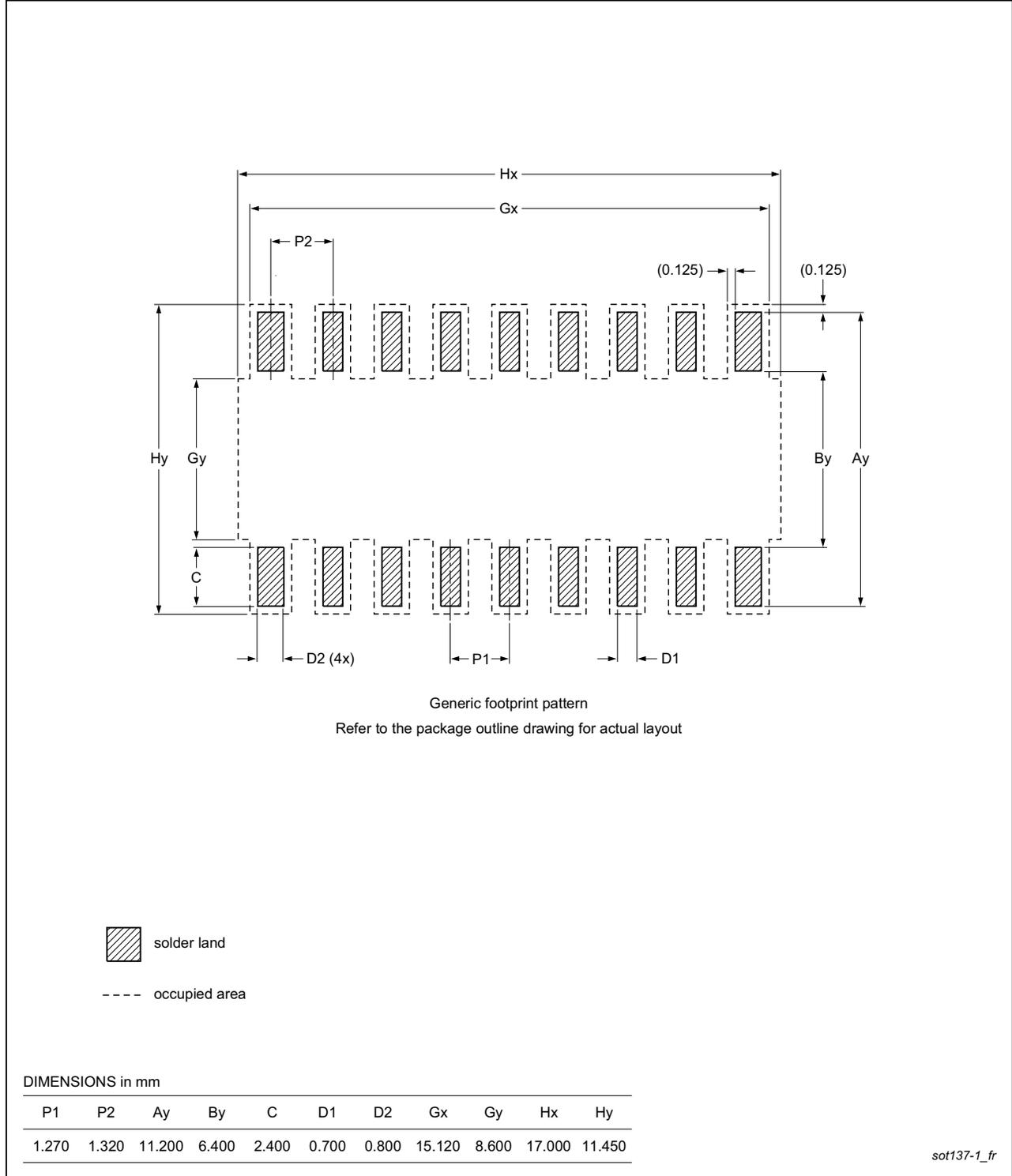
Fig 34. PCB footprint for SOT137-1 (SO24); reflow soldering
