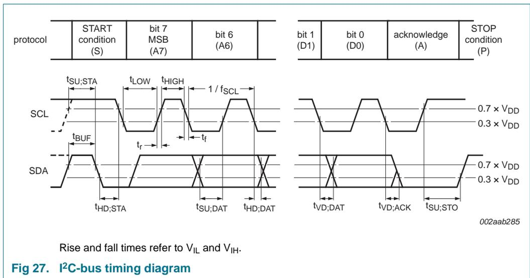
Fig 27. I<sup>2</sup>C-bus timing diagram
