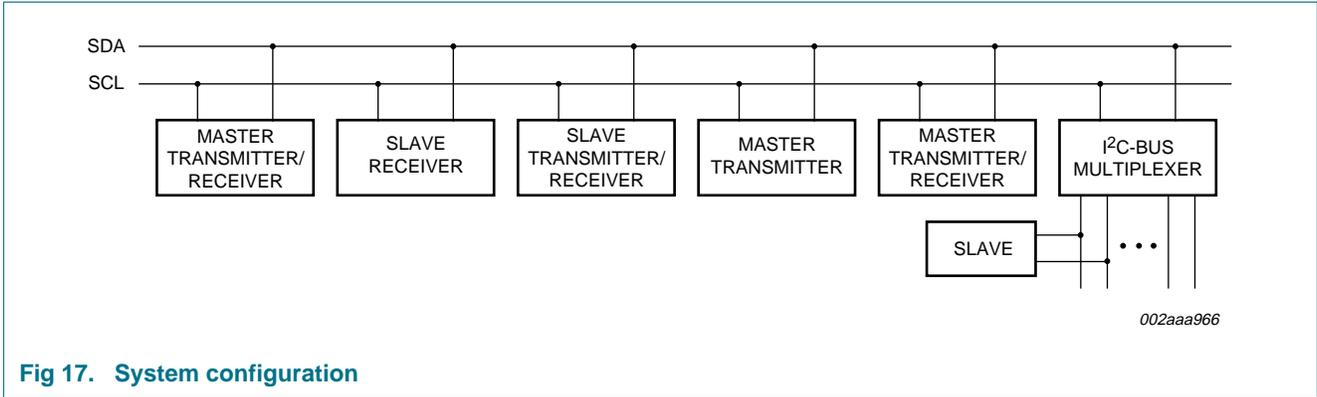
Fig 17. System configuration
