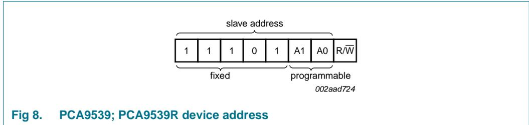
Fig 8. PCA9539; PCA9539R device address
