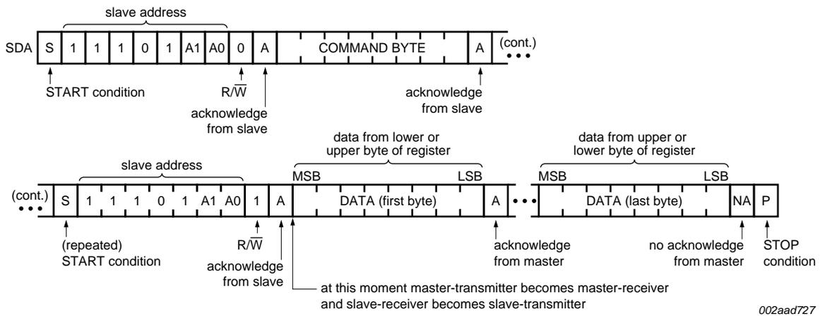
**Remark:** Transfer can be stopped at any time by a STOP condition.
