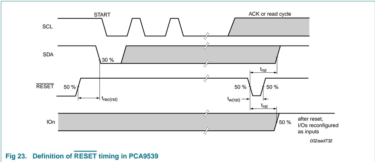
Fig 23. Definition of RESET timing in PCA9539
