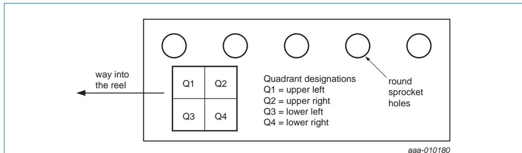
Fig 1. Carrier tape pin 1 quadrant designations
