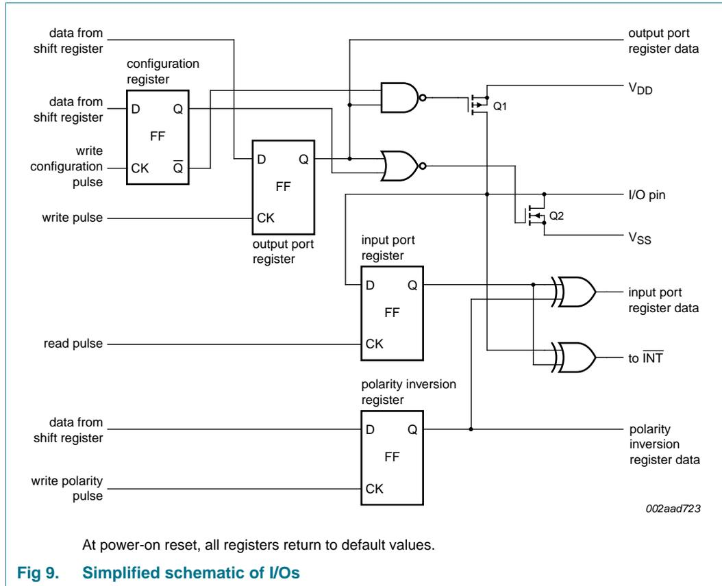
Fig 9. Simplified schematic of I/Os
