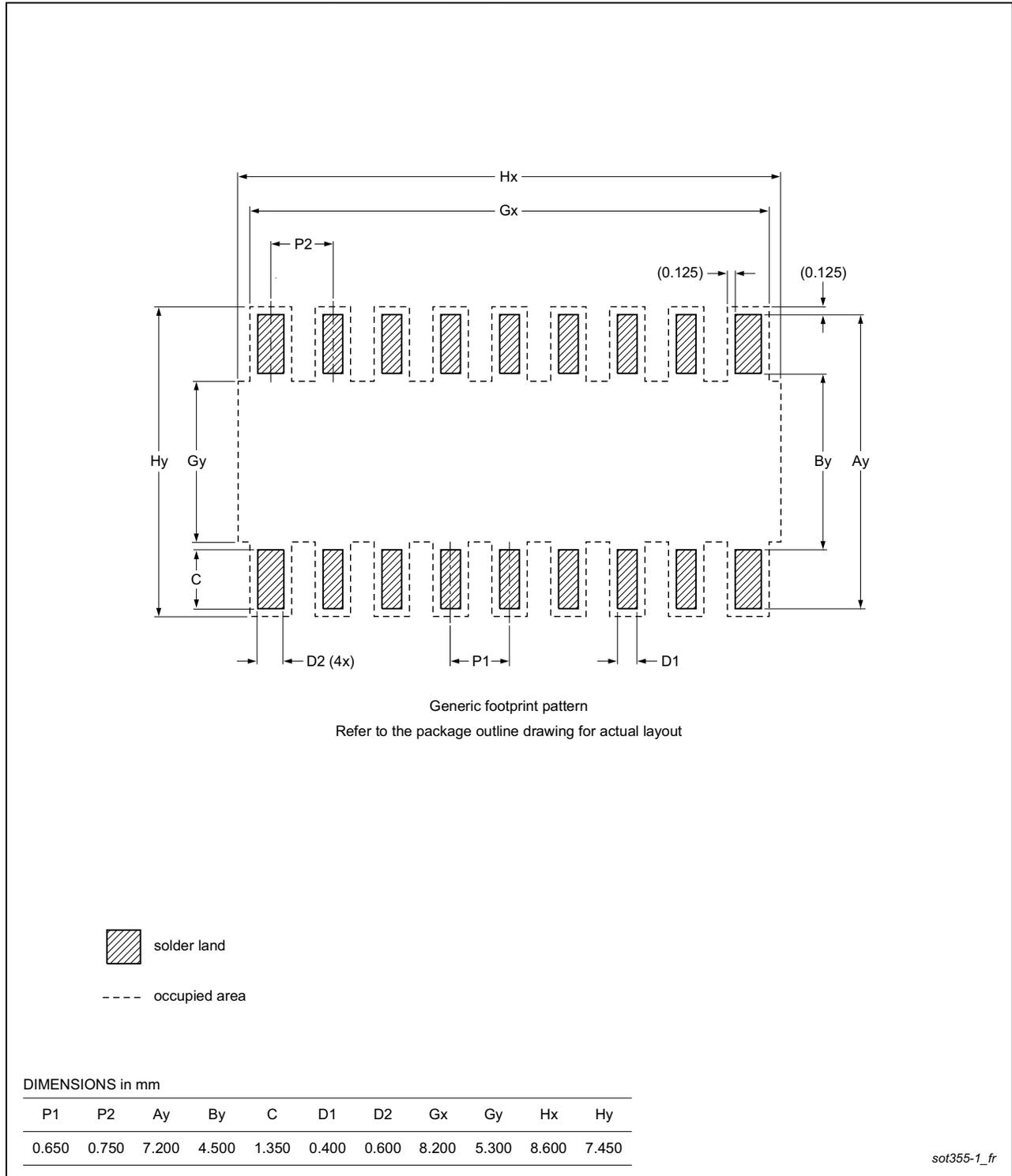
Fig 35. PCB footprint for SOT355-1 (TSSOP24); reflow soldering
