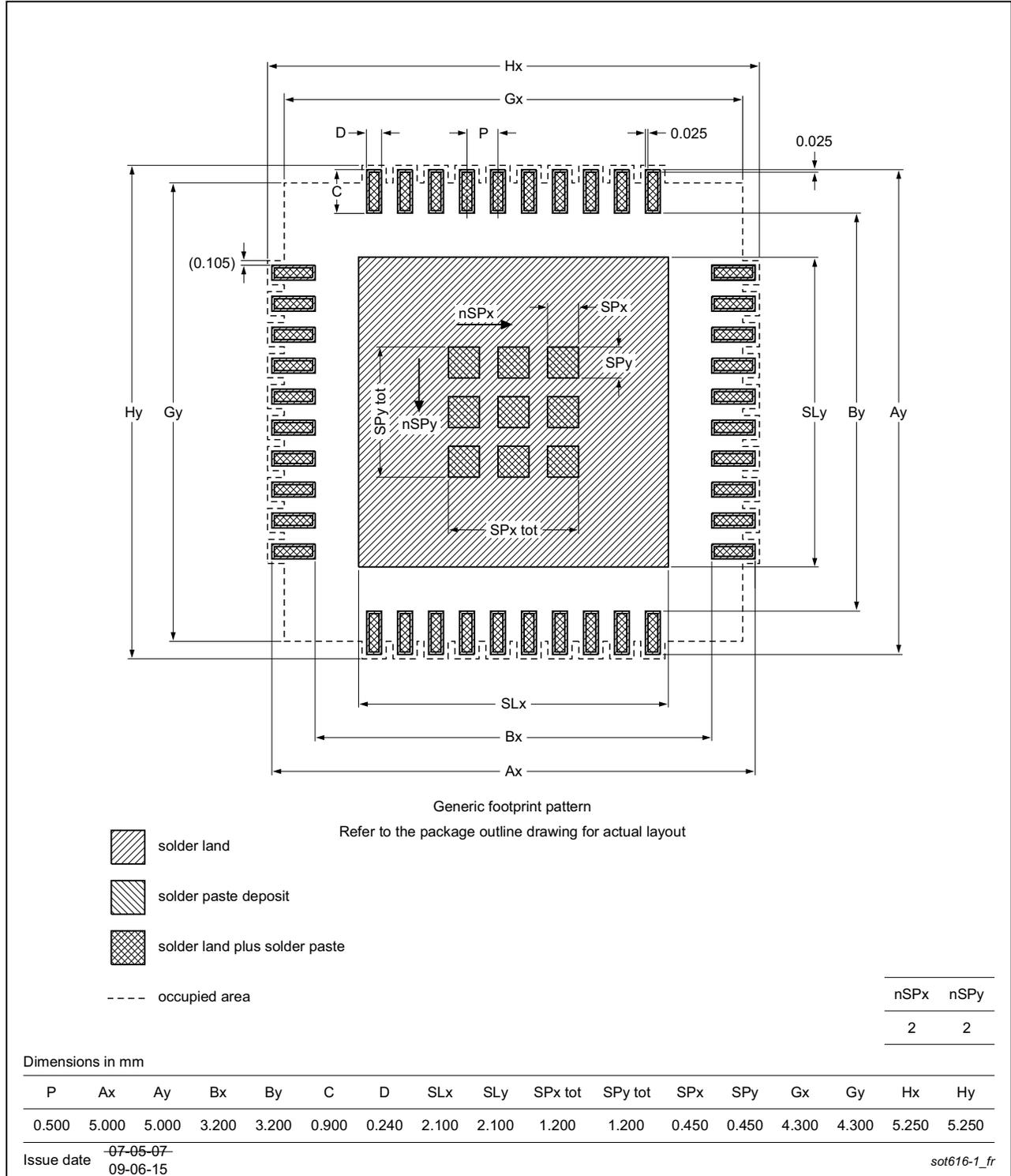
Fig 36. PCB footprint for SOT616-1 (HVQFN24); reflow soldering
