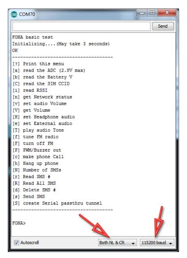
Make sure you also have **Both NL & CR** for the serial command sender option. This means when you send data to the Arduino via the console, it will put a newline/return at the end.
