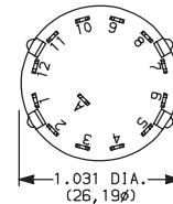
TERM. NOS. MOLDED ON HOUSING
