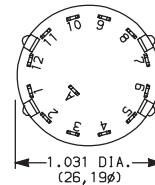
TERM. NOS. MOLDED ON HOUSING
