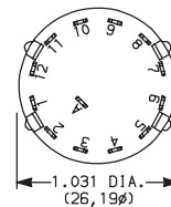
TERM. NOS. MOLDED ON HOUSING
