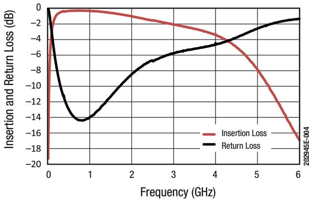
**Figure 4. Small Signal Performance without External Tuning**
