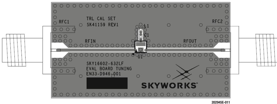
Figure 11. SKY16602-632LF Evaluation Board Assembly Diagram (Tuned Circuit)
