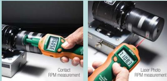
**Quickly measure RPM, surface speed and length with one tool. Use the contact wheel for up-close readings or laser mode for safer, non-contact measurements up to 1.6ft (0.5m) away.**
