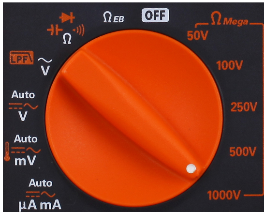
Figure 6. Insulation resistance tester with full featured DMM
