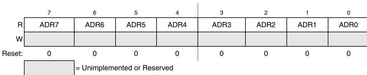
Figure 9-7. Data Result Low Register (ADCRL)
