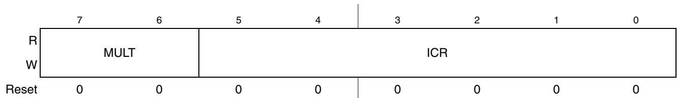
Figure 10-4. IIC Frequency Divider Register (IICF)
