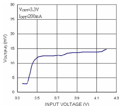
Fig. 24: V<sub>OUT</sub> Ripple Voltage for  $V_{IN}$  decreasing close to  $V_{OUT}$
