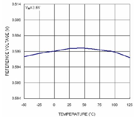
Fig. 9: Reference Voltage vs Temperature
