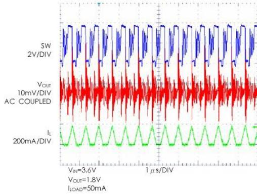
Fig. 16: Discontinuous Operation
