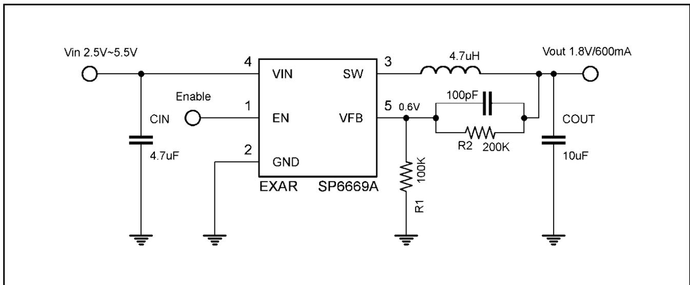
Fig. 1: SP6669 Application Diagram (Adj. version shown)
