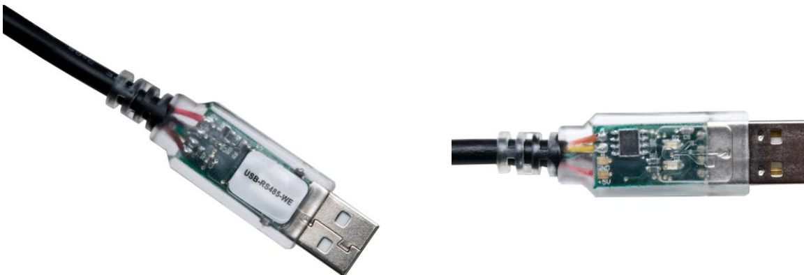
Figure 5.3 USB-RS485-WE Cable images
