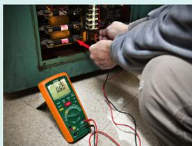
Checking voltage on a lathe
