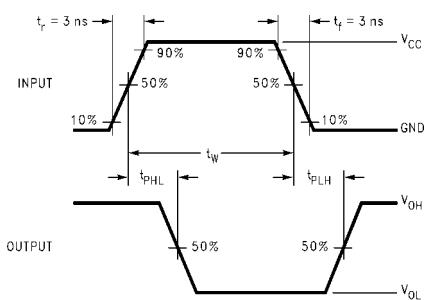
FIGURE 2. AC Waveforms
