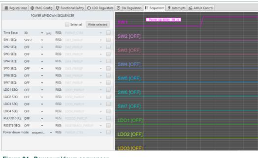
Figure 24. Power up/down sequencer
