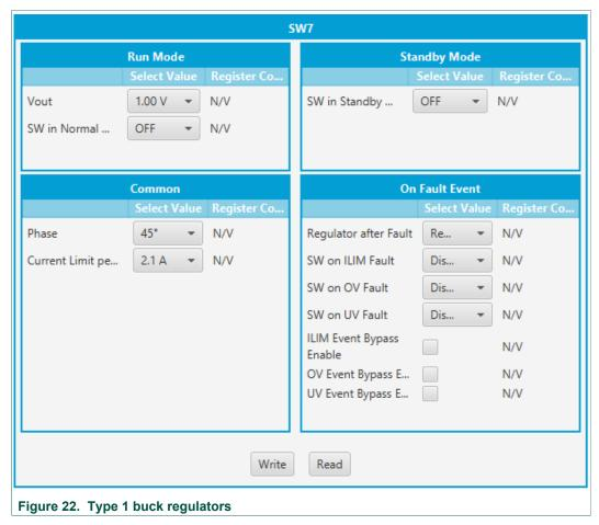
SW7 is a peak current mode controlled buck regulator operating in single phase only which provides higher output voltage settings typically used for 3.3 V I/O supply.
