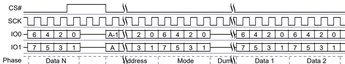
Figure 70. Dual I/O Continuous Read Command Sequence
